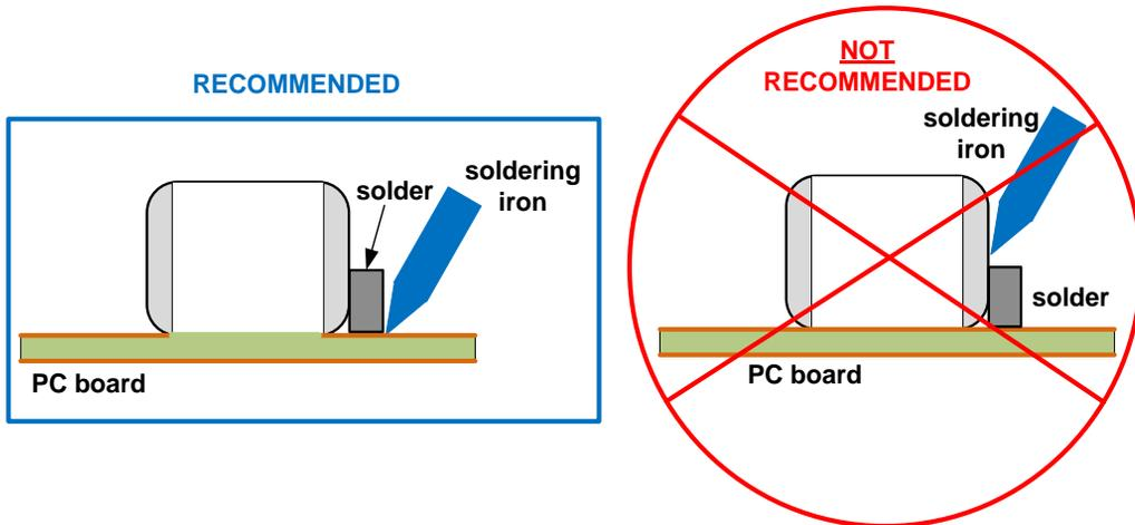
5. When a fillet forms, remove the iron. As shown in **Fig. 2**, solder fillets should occupy about 25-40% of the component's height, have a concave profile, and be free of peaks and voids.
